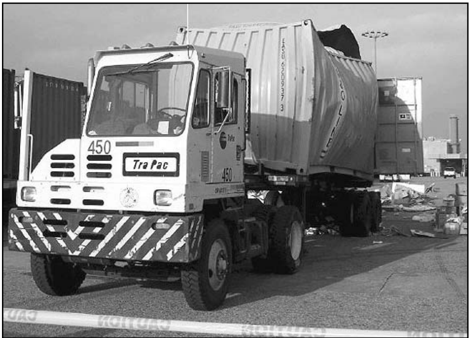
This is the container that slid onto the Tra-Pac terminal in the Port of Los Angeles without proper seals or documentation, and then exploded. If it had been loaded with the back doors facing the cab of the truck, the driver would’ve borne the full force of the blast.
