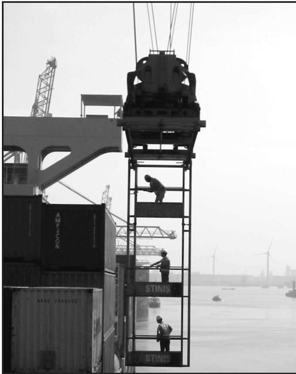
On the job in Rotterdam. Three longshore workers are lowered by a crane to remove twistlocks on the containers. The seven-high stack is too tall to be worked with lash sticks, so the lashers go over the side. The person on the top is a radio operator who stays in touch with the crane operator for safety reasons.
