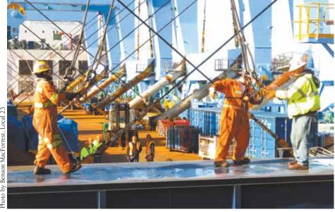
**Clearing the deck:** Several boxes were lifted to the dock, including water tanks used as counter weights to pull against. It all had to come off the deck to prepare for the discharge of the cranes themselves.
