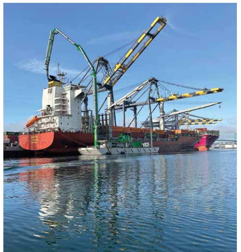
The Stax barge captures harmful emissions to reduce pollution. The newly-formed company currently operates in the Ports of LA and Long Beach but plan to expand to operate throughout California.
